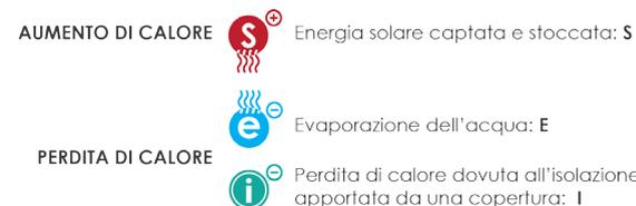
La Performance Energetica si misura in kW.h/mq: **PE = S-E-I**
